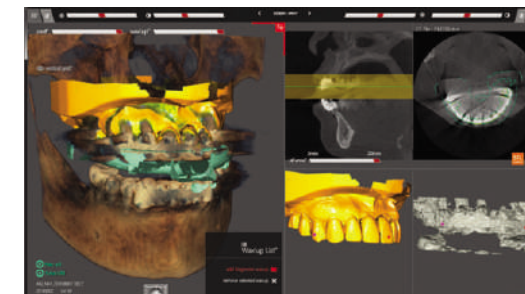
• Fig. 1. Superimposition process with CBCT using outline of radiographic guide tray of combination scan data.
