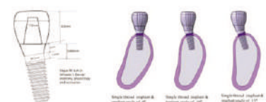
• Fig. 2. (Left) Design a dimension of restored prosthesis that cervical-occlusal is 8.5 mm and buccolingual is 7.5 mm according to Wheeler's dental anatomy, physiology and occlusion, (Right) Schematic drawing of the different implant angulation that is 0°, 10° and 15° in a bone.
